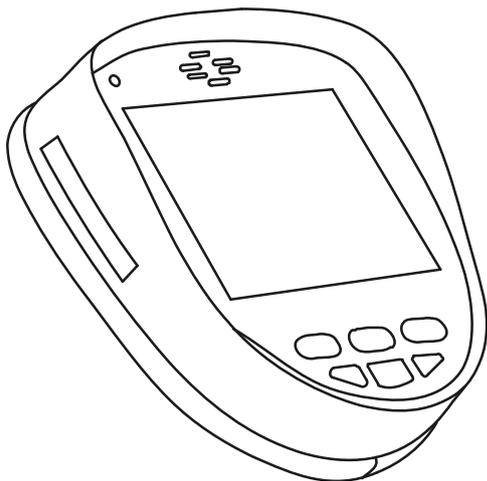
1. Open the protective rubber cover to access memory card slots
