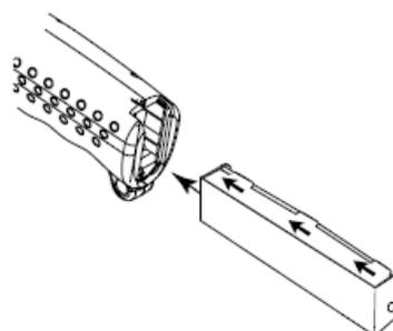
4. Insert battery cartridge into the handle and close the battery cover.
