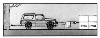
To double the pull, use 2-part line with snatch block and tie off to chassis. Take out of gear.
